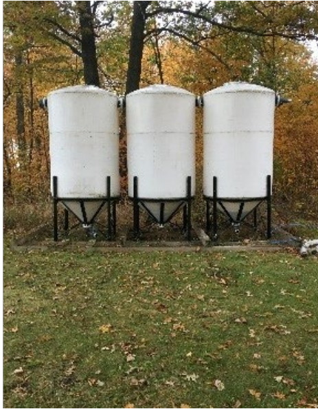
Figure 4.24 ERDC-EL 12-foot Sediment Collector™ System for Pilot Project
