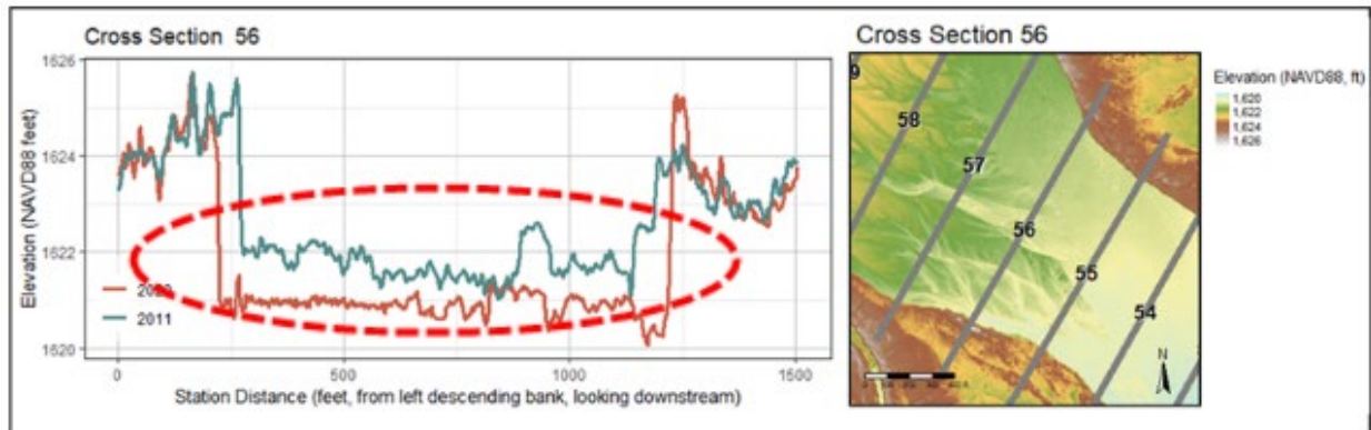
Figure 4.13 Niobrara River Channel Cross-section # 56 and Planview Upstream of Spencer Dam Site in Reach 14 Illustrating a Degrading Channel and Likely Location of Upstream Most Headcut
