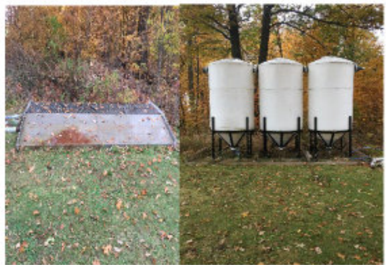
Figure 4. ERDC-EI 12-foot Sediment Collector™ system for Pilot Project
